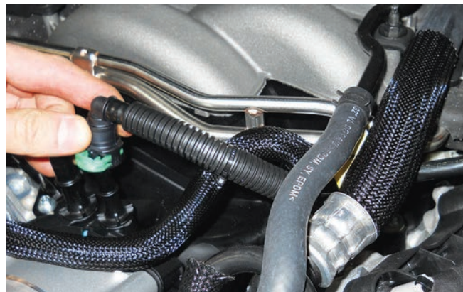
EECPV tube quick connector with green lock
