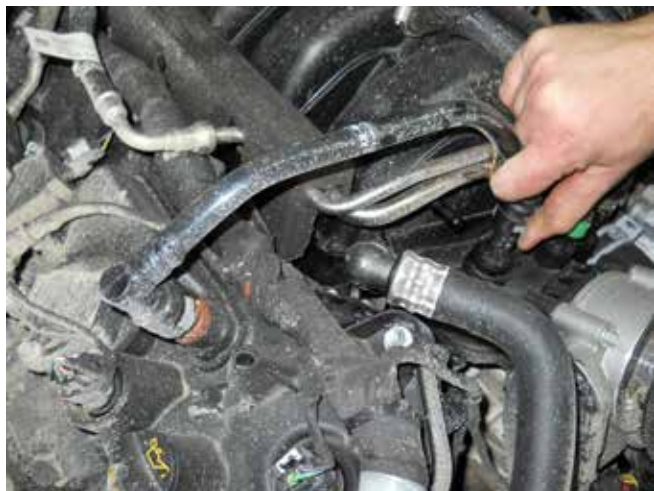
9. Disconnect the white quick-connect fitting from the brake booster.
