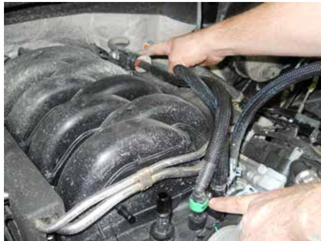
12. Disconnect the fuel supply line on driver side from the fuel rail. Refer to figure shown below. Use rags to catch fuel.
