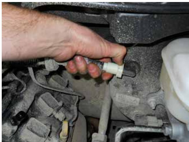
10. Disconnect the throttle body electrical connector. (Pull the red locking tab back; press the black release tab to disengage the lock.) Refer to figure shown.
