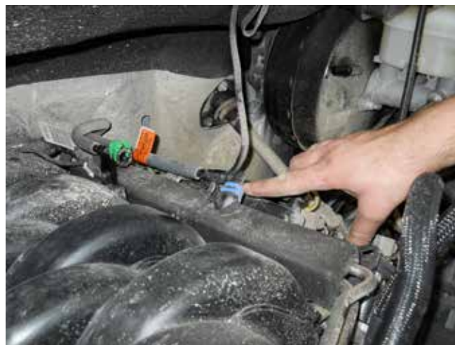
13. Use a 3/8" disconnect tool to disconnect the high pressure fuel line (RH side).
