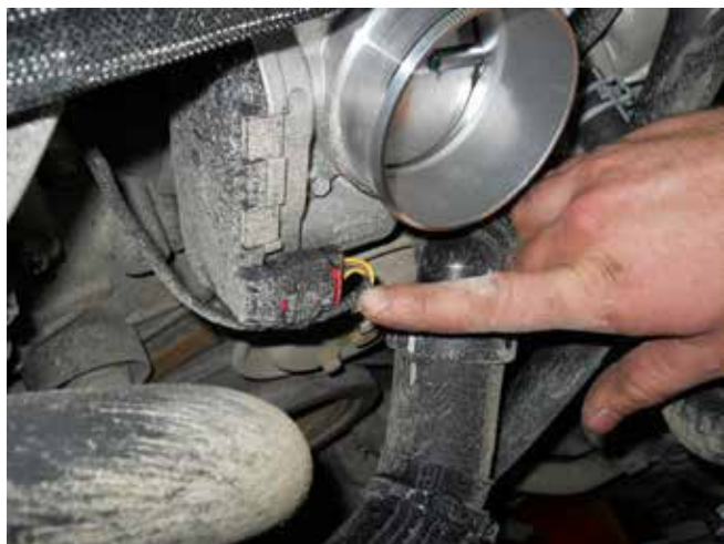
10. Disconnect the throttle body electrical connector. (Pull the red locking tab back; press the black release tab to disengage the lock.) Refer to figure shown.
